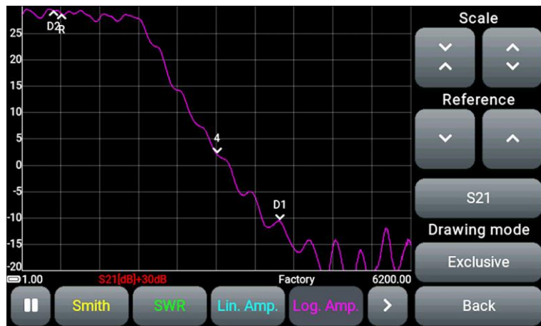
Figure 9.14 - Compensation of signal attenuation by attenuators
