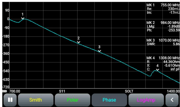
Figure 10.4 - Plot of the unwrapped phase in S11 measurement mode
