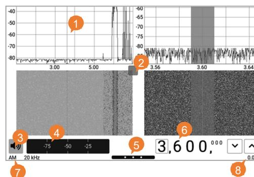
6.1. The instrument displays graphs of the spectrum / waterfall of the bands of interest. The current settings and interactive buttons for controlling the instrument interface are located at the bottom of the screen.
